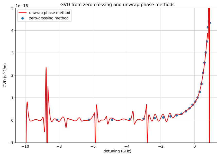
Figure 14: Example of an oscillating estimation of the GVD caused by a wrongly chosen smoothing factor s . The data used is the same as in figure 13.
